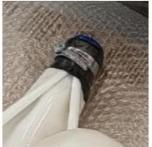
The Silicone bladder is wrapped in and fixed with insulation tape. Which also serves as a protection for the silicone hose. Then tightened tightly with a hose clamp.
